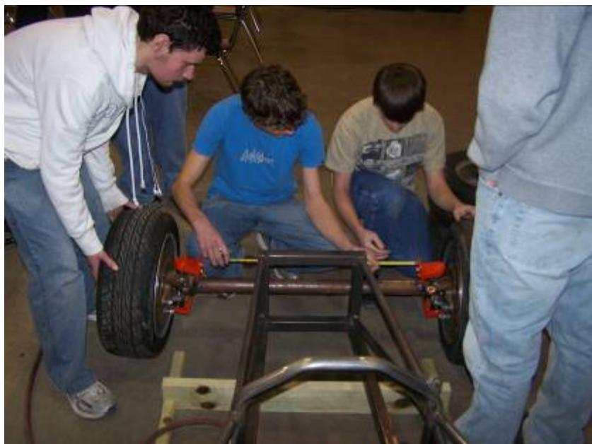
The next challenge Team 1 faced was to mount and align the steering system. About a dozen designs were thrown around, until finally it was decided to just use the simplest and most effective one. This was to weld a 4" tube onto the axle, then weld a bracket on the other end of the tube, and bolt the system into the bracket. This whole process took nearly an hour, most of which was spent measuring and centering.
